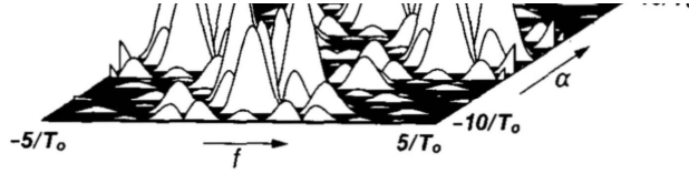
Fig. 7. Spectral correlation magnitude surface for Manchester-encoded binary phase-shift keying with carrier frequency = 3.3/T_0 .
