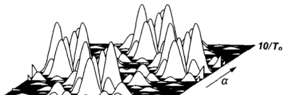
Fig. 6. Spectral correlation magnitude surface for minimum-shift keying with carrier frequency = 3.3/T_0 .
